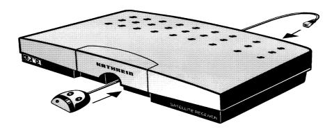
The movable infra-red sensor receives the remote control signal and feeds it through the cable into the receiver. Naturally the movable sensor may be placed apart from the receiver. In order to save space, the receiver may be positioned any where within sight and range of the remote controller.
